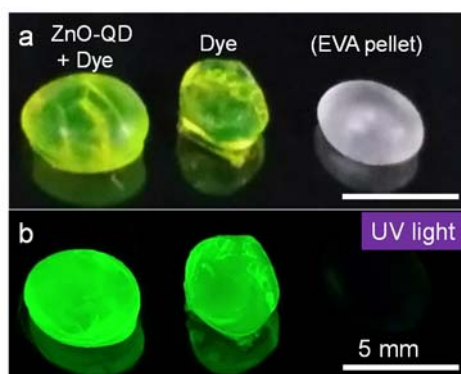
Fig.1 Photos of EVA pellets under (a) white light and (b) mercury lamp.
