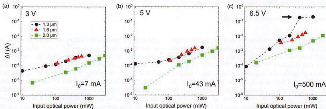
**Fig. 2.** (Color online) The dependence of changes in the output current on the incident light intensity: (a)–(c) indicate results of applying the forward voltage to the device at 3 V, 5 V, and 6.5 V, respectively. Here,  $I_0$  in the figure shows the value of the forward current without incident light beams. In addition, the individual plots indicate the wavelengths of the incident light beams.
