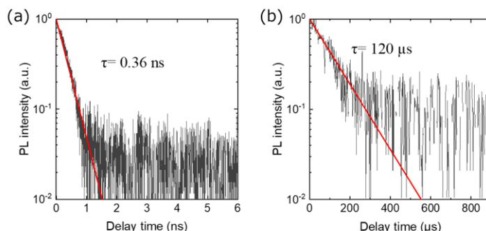
Fig.2 Decay curve of time resolved measurements. (a) DP Si-LED. (b) Si p-n crystal.
