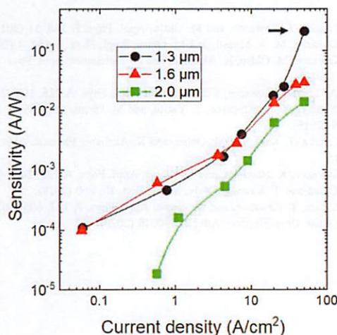
**Fig. 3.** (Color online) The photosensitivity with respect to the injection current density. The individual plots indicate the wavelengths of the incident light beams.
