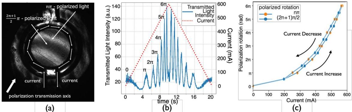
Fig. 1 (a) Transmission image of SiC-SLM with polarized light (b) Variation of transmitted light intensity as a function of time (current) (c) Polarization rotation angle as a function of current.
