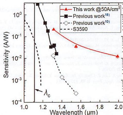
**Fig. 4.** (Color online) Comparisons with the previous work for the photosensitivity with respect to wavelength. For the present study, the results are shown for a forward current density of  $50 \text{ A cm}^{-2}$ .
