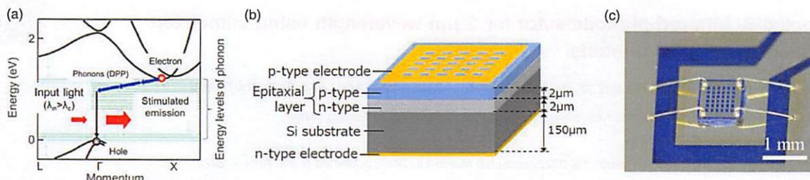
**Fig. 1.** (Color online) The structure of Si infrared photodetector: (a) band diagram of Si for describing the operating mechanism of the present device; (b) schematic diagram of the device structure of the present device; and (c) micrograph.
