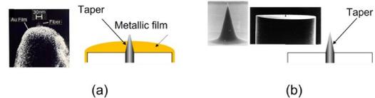
Fig.1 External forms and cross-sectional structures of the fiber probe. (a) A high-efficiency fiber probe. (b) A basic fiber probe.
